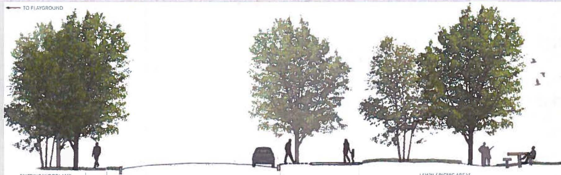
EXISTING WOODLAND 5' PATH 2' TURF 35' 8TH STREET SOUTH VARIES PAVING WITH COBBLE DETAIL AROUND TREES LAWN / PICNIC AREAS SECTION D-D' 8TH STREET SOUTH ENHANCED SIDEWALK SCALE: 1" = 5'
