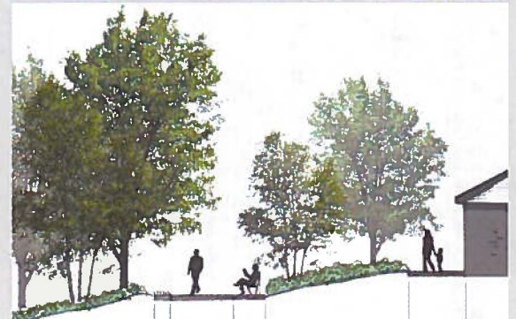
EXISTING WOODLAND WITH UNDERSTORY PLANTING 2' FIBER SOILS 3' BENCH PAD VARIES SLOPED PLANTING 10' PATH REST ROOM SECTION E-E' RESTROOM FRONTAGE SCALE: 1" = 5'
