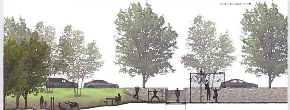
EXISTING WOODLAND WITH UNDERSTORY PLANTING 6' PATH VARIES ATHLETIC SURFACE VARIES LAWN ACTIVITY SPACE 6' PATH BASKETBALL COURT SECTION B-B' BASKETBALL COURT SCALE: 1" = 5'
